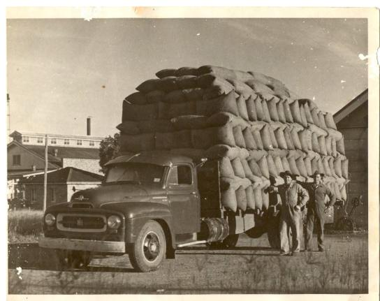
A load of peanuts waiting at the Proston Railway Station to be loaded on a train bound for the Peanut Board in Kingaroy. The truck, a 162 International, was owned by Clive Latcham (front) and driven by Norm Smoothy (behind) and could carry between 400 and 500 bags of peanuts. These peanuts were grown on Bert Graham's property at Farmer's Road, Abbeywood. Photo taken in 1957.
